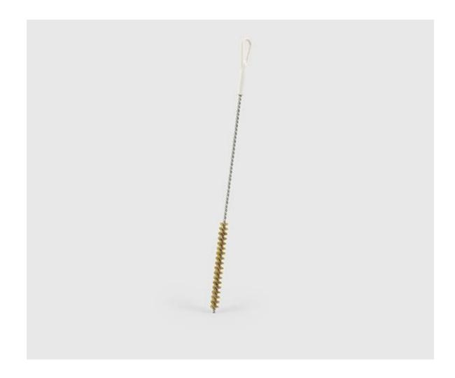
$120 \text{mm} \times 13 \text{mm} \emptyset$  (400 mm overall) Twisted in wire tube brush, made with mild steel galvanized wire, filled with bristle with a white Polypropylene handle fitted. Bristle tends to have more give than plastic, and is not as aggressive.
