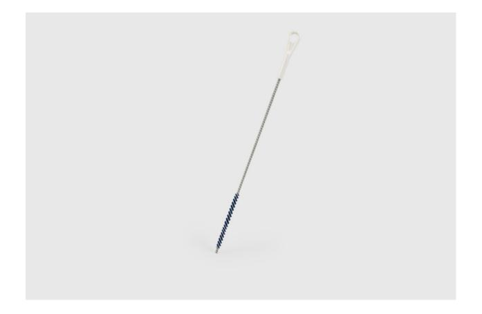
120mm x 10mmø (400mm overall)Twisted in wire tube brush, made with mild steel galvanized wire, filled with Polyester PBT, blue only fitted with white Polyproplene handle. Polyester will distort at temperatures of 130°C.
