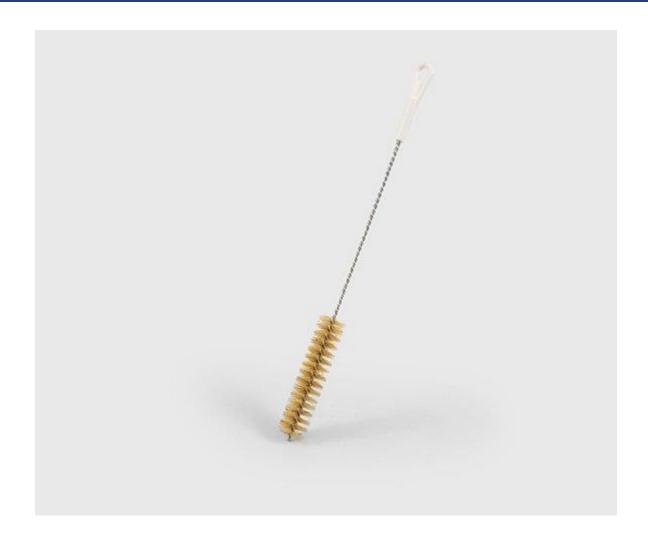
105mm x 31mmø (400mm overall) twisted in mild 14g steel galvanized wire tube brush, with fan tuft, filled natural bristle and fitted with white Polypropylene handle. Natural bristle is soft while resilient, and is particularly good for cleaning glass.
