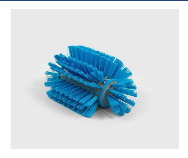
216mm overall length x 137mm wide tank brush, Polypropylene block filled medium Polyester, Resin-Set DRS®, for cleaning tanks, vats and gullies. The material covers 360 degrees, and the only side not filled is where the handle fits. Recommended handles, ALH27 or ALH8. A softer version is available, D77RES.
