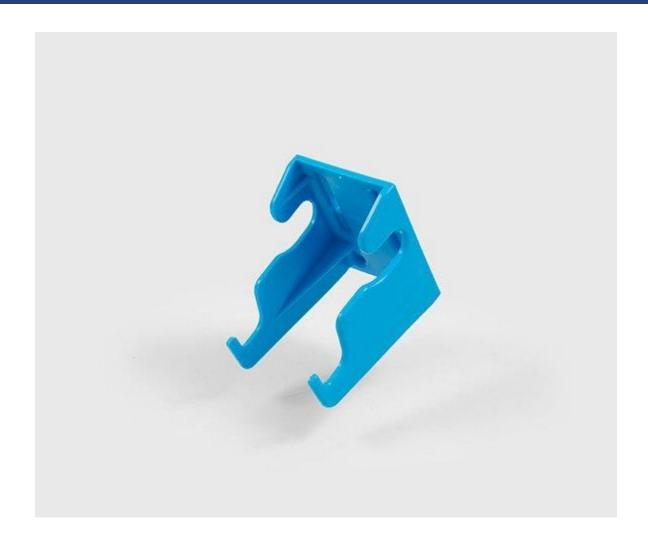
Plastic wall bracket for both hanging up the HH1 at 90° to the wall for use if desired, or flat against the wall for storage, or for storing the MBK15 bucket. Approximate dimensions, 83mm wide x 108mm deep x 121mm out. Keyhole slots allow easy installation and removal. Fixing screws are not included.
