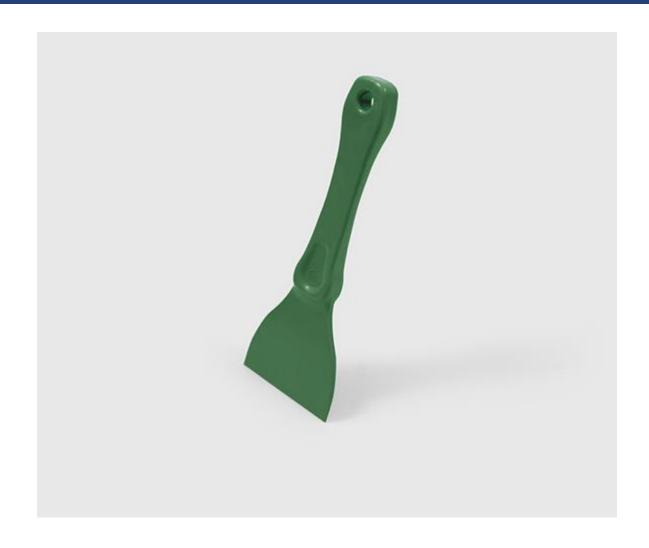
76mm wide Polypropylene hand scraper, 205mm long, with hanging hole. This scraper is very good in normal use on smooth surfaces. For very stubborn, hard, stuck-on debris consider the stainless steel MSC22 or MSC3/38. See also the larger PSC2, and the FLPSC3.
