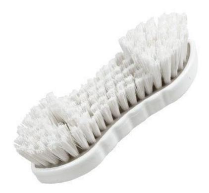
210mm two level scrub, Polypropylene block, filled stiff Polyester, Resin-Set DRS<sup>®</sup>. This is a most effective heavy duty hand scrub. By pushing down hard during scrubbing action, the filaments at the ends of the brush splay out, getting into hard-to-reach corners. The block has a comfortable grip. See also ST5RES, ST7.
